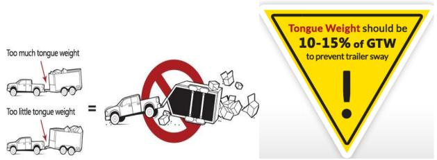
proper towing tongue weight should be no less than 10 percent of gross trailer weight (GTW) and no more than 15 percent. For example, tongue weight for a 10,000 pound trailer should be no less than 1000lbs, and no more than 1500lbs.
