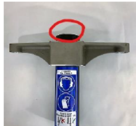
INCORRECT POSITION OF THE BOTTOM HAMMER STEM FROM NOT MAINTAINING DOWNWARD PRESSURE ON THE MACHINE
