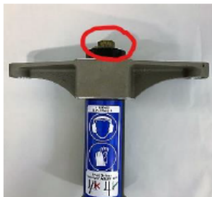
CORRECT POSITION OF THE BOTTOM HAMMER STEM FROM MAINTAINING THE DOWNWARD PRESSURE ON THE MACHINE
