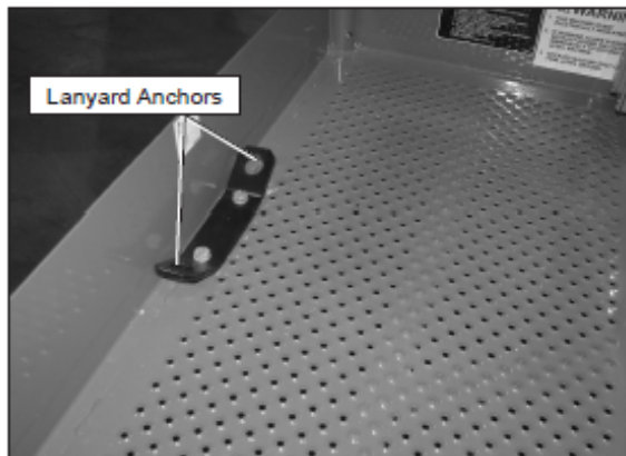
Figure 8.16 – Inside Rear of Platform
