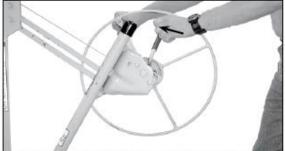
To lower the PANELLIFT\* Drywall Lift control the backward rotation of the winch by grasping the winch handle with your right hand BEFORE releasing the brake with your left hand. ALWAYS use this two hand method when lowering the PANELLIFT\* Drywall Lift.  The PANELLIFT\* Drywall Lift will hold drywall in position on sidewalls and sloped ceilings in addition to level ceilings. The cradle also tilts up to 10° longitudinally.
