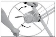
To raise the PANELLIFT\* Drywall Lift rotate the winch wheel in the direction shown. The brake arm is spring loaded to hold the winch automatically at any height.
