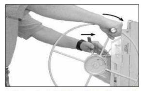
To move the winch into the working position rotate the winch forward slightly with your right hand while raising the brake arm with your left hand.
